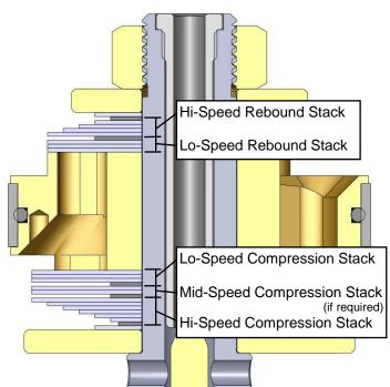
NOTE: All measurements are metric (for inches divide by 25.4). The valving list starts at the piston face and goes towards the base plate. Valve specs are listed by (QUANTITY) THICKNESS x DIAMETER. Example: (2).20x40 means quantity two, 20 hundredths of a millimeter thick by 40 millimeters in diameter.
